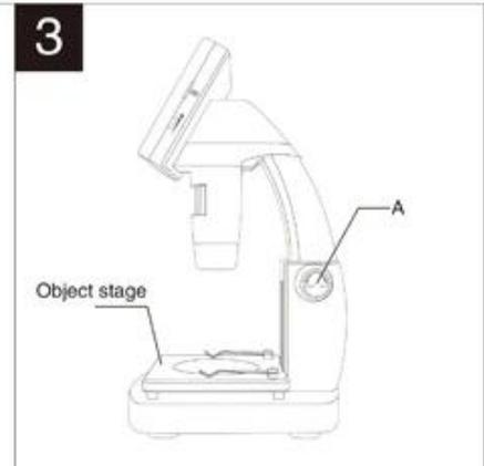
3. Put object to be observed onto the object stage, Rotate Wheel A to bring the object near to the microscope tube.
