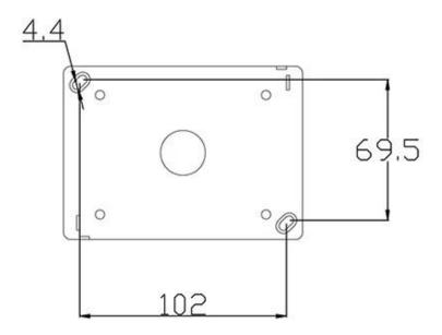
Material:Plactics,White Ingress Protection:IP55 Size:118\*86mm Suitable for two British wall sockets How to Install
