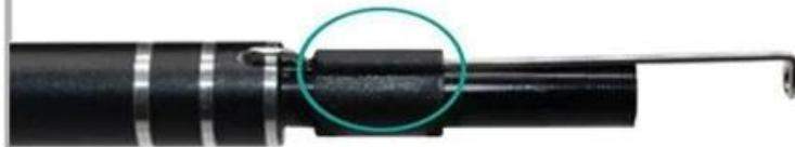
3. Push the fixing sheath to the bent part of the ear scoop.
